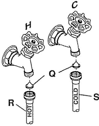
Determine which is **HOT** water line before attaching water hoses to faucets. Traditionally, **HOT** faucet is on left.
