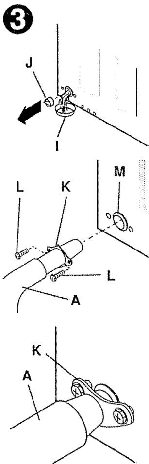
**3** Place a cooking dish or pan **I** under drain opening on back of washer. Pull plug **J** out of grommet **M** with pliers and discard. Water left over from factory test will drain. Remove container **I** and water.
