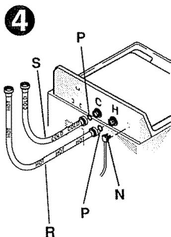
**4** Remove electrical cord **N** from storage before installing water hoses. Install rubber washer **P** in one end of hot water hose **R**. Thread hot water hose **R** onto connection labeled **H** at top rear of washer. Hand tighten, plus an additional 1/8 turn with pliers.
