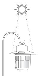
BEFORE FIRST USE – Pull out to remove the clear plastic strip with orange sticker in the light fixture to charae batteries.
