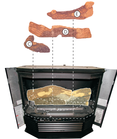
Log Placement Figure 43
