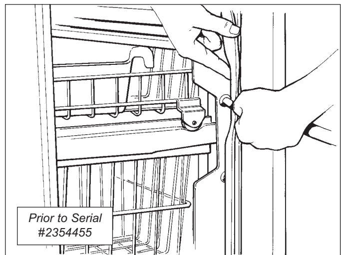
Figure 2-10. Drawer Front Pitch Adjustment
