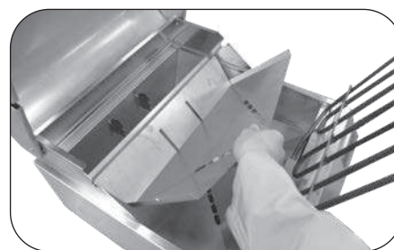
Fig. 22-4 Remove rear liner
