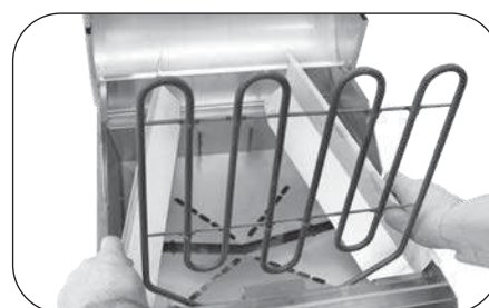
Fig. 22-3 Remove side liners
