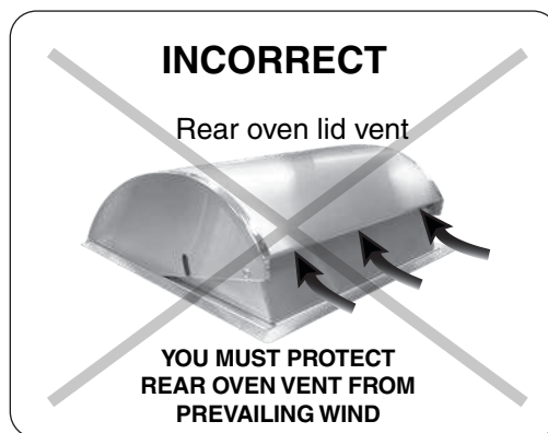
Fig. 8-3 Airflow direction - INCORRECT
