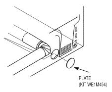
Connect standard metal elbows and ducts to complete the exhaust system. Cover back opening with a plate (Kit WE1M454) available from your local service provider. Place dryer in final location.
