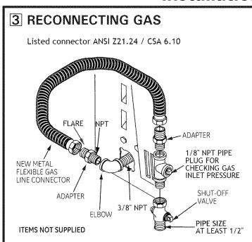
Note: The connector and fittings are designed for use only on the original installation and are not to be reused for another appliance or at another location. Keep flare end of adaptor free of grease, oil and thread sealant.
