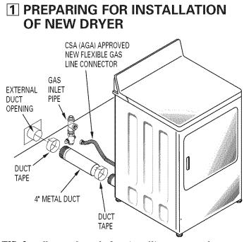
TIP: Install your dryer before installing your washer. This will allow better access when installing dryer exhaust.
