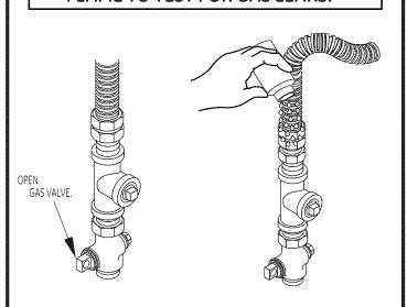
Check all connections for leaks with soapy solution or equivalent. Apply soap solution. Leak test solution must not contain ammonia which could cause damage to the brass fittings. If leaks are found, close valve, retighten the joint, and repeat the soap test.
