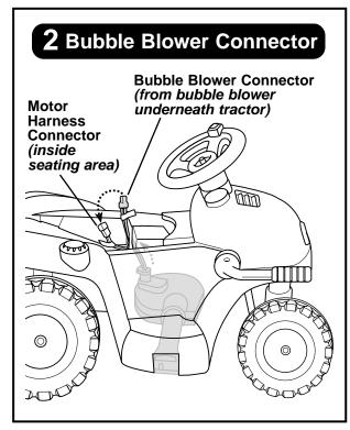
Next, connect the bubble blower connector (labeled Bubble Blower) to the second motor harness connector (labeled Bubble Blower) inside the seating area of the tractor.
