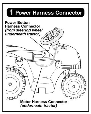
You must first connect the steering wheel power button harness connector to the motor harness connector underneath the tractor. Please refer to Assembly steps 10 and 11 on page 10 in your Owner's Manual.
