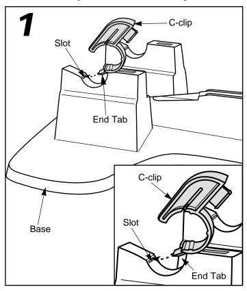
• Insert the end tab on a C-clip into the slot in the base.
