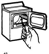
**Before** replacing the light bulb, be sure to unplug the **dryer power** cord or disconnect the dryer at the household distribution panel by removing the fuse or switching off the circuit breaker. Reach above **dryer** opening from inside the drum. Remove the bulb and replace with the same size bulb.
