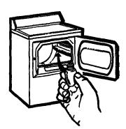
**Before** replacing the light bulb, be sure to unplug the **dryer power** cord or disconnect the dryer at the household distribution panel by removing the fuse or **switching** off the circuit **breaker.** Reach above **dryer** opening from inside **the** drum. Remove the bulb and replace **with** the same **size** bulb.
