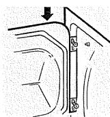
Rotate the door 180°. Insert it on the opposite side of the opening by moving the door IN and DOWN until the top hinge and the bottom hinge are resting on the top screws inserted in step 1.
