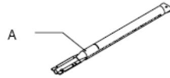
A. Air shutter adjustment screw
