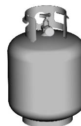
LP cylinder in upright position for vapor withdrawal
