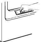
**Stainless Steel:** To clean stainless steel surfaces, use a damp cloth with a mild, non-abrasive cleaner suitable for stainless steel surfaces. Remove the cleaner residue, and then dry with a clean cloth.
