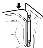
Rotate the door 180°. Insert it on the opposite side of the opening by moving the door *IN* and *DOWN* until the top hinge and the bottom hinge are resting on the top screws inserted in step 1.
