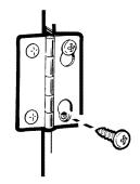
Remove the remaining screws from the side of the opening from which the door was removed. With these screws, secure each hinge at the bottom. Tighten the 2 top screws of each hinge. Reinsert the plastic plugs on the side from which the door was removed.
