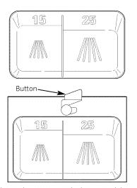
To open the wash cover, press the button and the cover will flip back.
