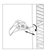
Loosen hex nut on door latch. Turn hook clockwise to tighten as shown.
