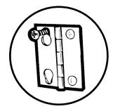
Loosen top screw from each hinge on the dryer face half way. With one hand holding the top of the door and the other hand holding the bottom, remove the door from the dryer by lifting it *UP* and *OUT*.
