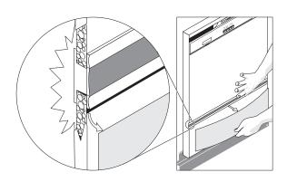
8. Replace bottom trim by fitting slot over bottom edge of door and secure by pressing from one side to the other. **Note:** If trim does not go on easily, check to make sure assembly is pushed all the way up under the control panel and spacers and panels are in channel of divider trim strip.
