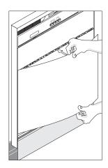
Move complete panel assembly up by pushing from sides and bottom of lower panel. Check to make sure the color panel(s) fit securely under control panel by pressing in at top of color panel(s).
