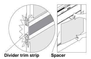
4. Check to see if spacer has remained in the channel of the divider trim strip. If it has not, replace securely in channel. It may be helpful to gently push in on divider trim strip while reinserting the spacer.
