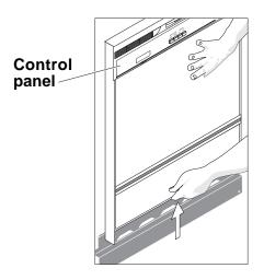
7. To change lower panel, use one hand to hold upper panel assembly and divider trim strip in place and use the other hand to slide lower panel down until it clears divider. Remove panel(s), arrange desired color and replace per above directions for upper panel. Do not remove foam spacer.
