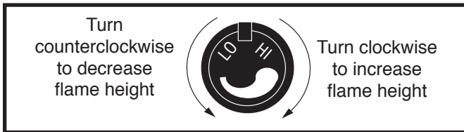
Fig. 56 Flame adjustment knob for Honeywell valve.
