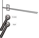
Note: Hot water needs to be at a temperature of at least  $120^{\circ}$  F -  $140^{\circ}$  F. (49° C- 60° C) for the soap to dissolve and to avoid soap residue remaining on clothes.
