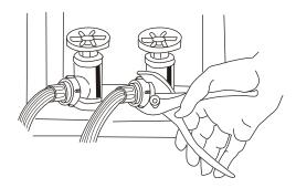
2. Connect the hot and cold water inlet hoses to the hot and cold water faucet.
