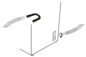
5. Plug in the Washer to a regular 115 volt / 60 Hz, 15 amp outlet.
