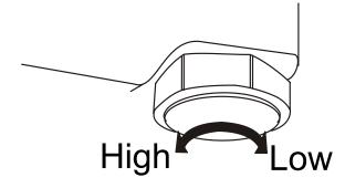
Warning: Leveling of washer is very important to prevent vibration during spin.
