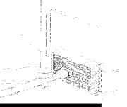
DO NOT touch the condenser fins. They are sharp and can be easily damaged.
