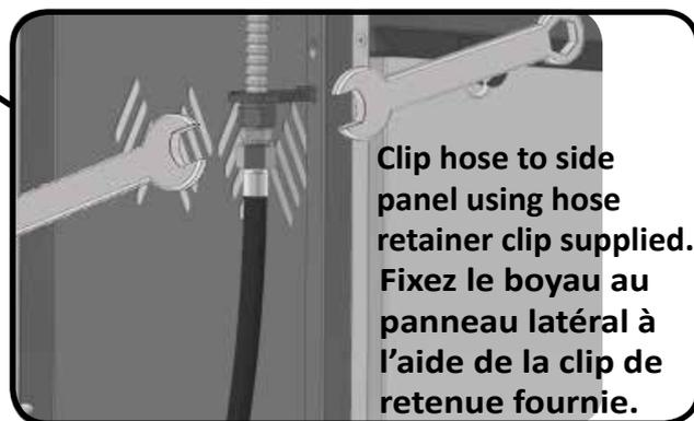
Clip hose to side panel using hose retainer clip supplied.
