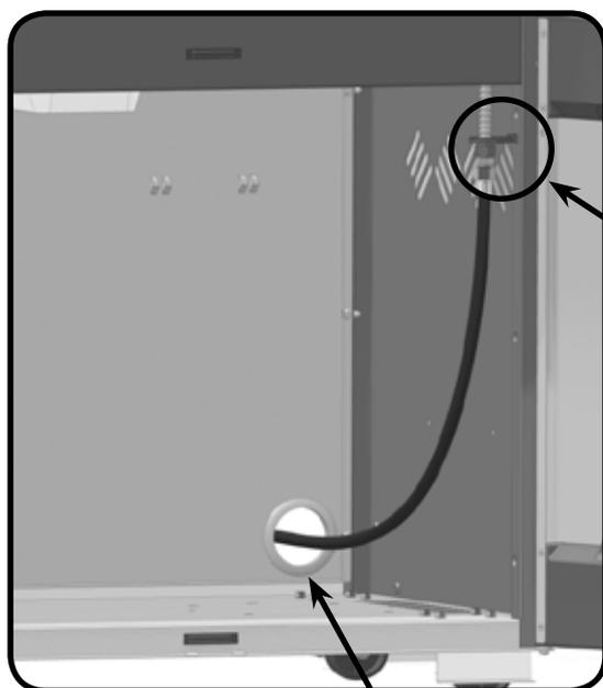
Bushing is pre-installed at factory.
