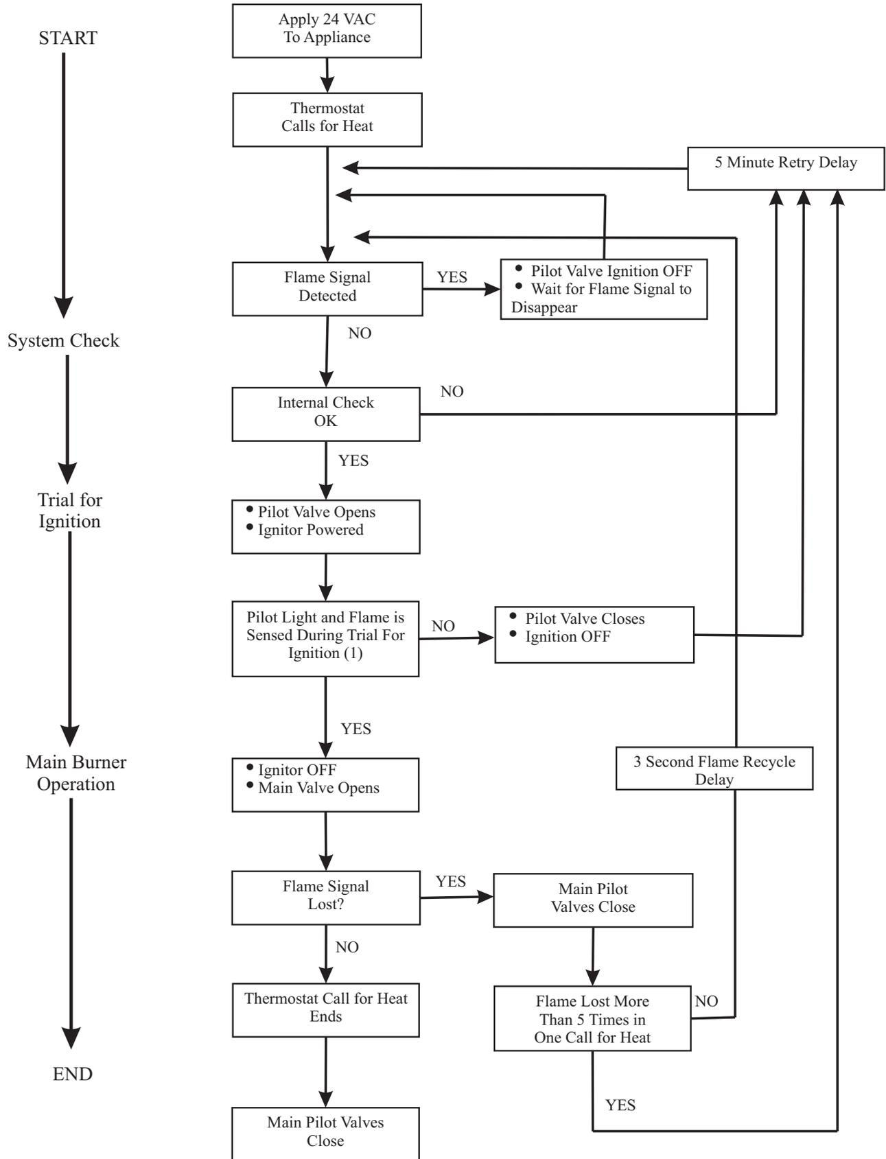
(1) Ignitor will turn OFF about 30 seconds into the trial for ignition if the pilot flame has not lit. It will turn back ON for the final 30 seconds of the 90 second trial for ignition. The pilot will be energized during the entire trial for ignition. This is normal operation for this gas ignition system.
