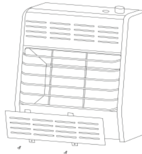
Figure 7 - Removing Lower Front Panel Of Heater
