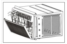
The air filter should be checked at least once a month to see if cleaning is necessary. Trapped particles in the filter can build up and cause an accumulation of frost on the cooling coils.
