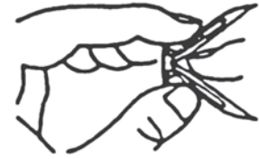
Fig. 17 - Folding the Expansion Bracket
