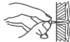
Fig. 19a - Attaching Wall Hanging Spacers to Heater
