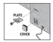
Check and clean off any debris from the fan air intake vent, found on the bottom of the hopper. Once the hopper access
