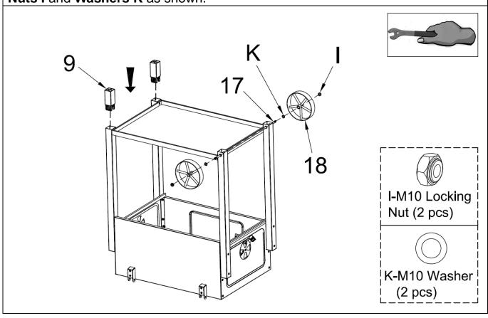
**Step 8.** Tighten the bolts in steps 1 and 5.
