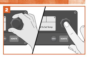
To select temperature, turn Selection dial right or left; once desired temperature is displayed, press the center of the dial to select.
