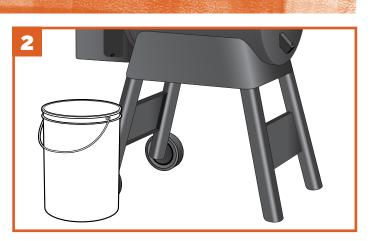
Place a container large enough to hold the discarded pellets under the pellet clean-out door.
