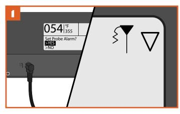
Plug the probe into the probe jack located on the WiFIRE<sup>®</sup> Controller. The controller will recognize the probe and the probe icon will light in the controller screen's upper-right corner. The display will ask if you want to set an alarm. Select YES.
