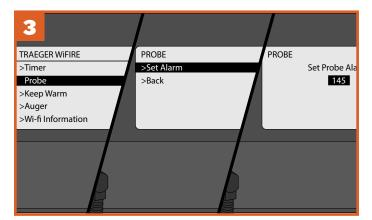
Press MENU; then scroll and select PROBE. You will be prompted to set a probe alarm for the internal goal temperature. Select SET ALARM. Then, at the probe menu, use the Selection dial to choose the temperature goal for your meat.
