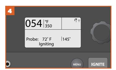
Once the probe alarm is set, the home screen will display the grill temperature, goal probe temperature, and grill status. A tone will sound when your meat reaches the set alarm temperature. If using the Traeger WiFIRE<sup>®</sup> app, you will receive a push notification on your connected smart device, along with a display of your grill's status throughout the cooking process.
