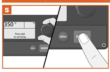
The home screen will display "Press dial to set temp." Turn the Selection dial clockwise to 350°F (177°C). Press IGNITE, close grill door, and run grill for 20 minutes once it has reached the set temperature.
