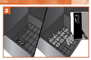
Make sure there are no foreign objects in the auger before adding pellets to the hopper.
