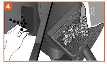
Once the hopper's empty, close the door, replace the fastener, and refill the hopper with a different flavor of TRAEGER<sup>®</sup> BRAND HARDWOOD PELLETS.
