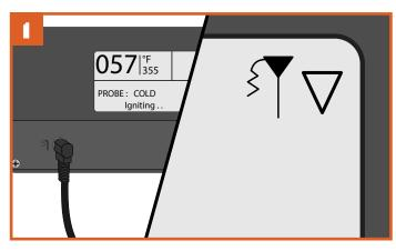
Plug the probe into the probe jack located on the WiFIRE<sup>®</sup> Controller. See "Using Your Grill" to turn on the grill. Once the grill is on, the controller will recognize the probe and the probe icon will light in the controller screen's upperright corner.
