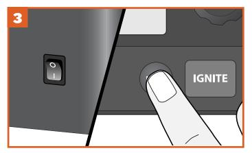
Turn grill on: Flip the Main Power switch on the back of the grill to ON (I), **press any button on the control panel to activate** the WiFIRE<sup>®</sup> Electronic Controller. After a few seconds, the home screen will display.
