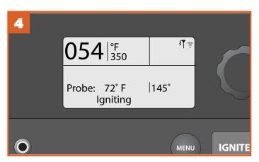
Once the probe alarm is set, the home screen will display the grill temperature, goal probe temperature, and grill status. A tone will sound when your meat reaches the set alarm temperature. If using the Traeger WiFIRE® app, you will receive a push notification on your connected smart device, along with a display of your grill's status throughout the cooking process.
