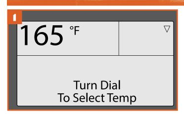
After turning ON (I) the Main Power switch, your grill's home screen defaults to the "Turn Dial To Select Temp" message. Cooking temperature can be set directly from this screen.
