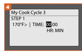
If the recipe calls for a specific number of hours at a set temperature, select TIME. To select hours, rotate the dia Press to select and move to minutes. Rotate to choose minutes and press the dial to select and finish.
