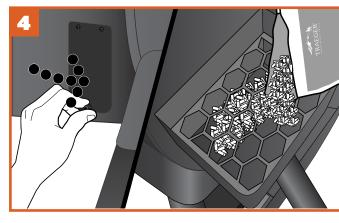
Once the hopper's empty, close the door, replace the fastener, and refill the hopper with a different flavor of TRAEGER<sup>®</sup> BRAND HARDWOOD PELLETS.
