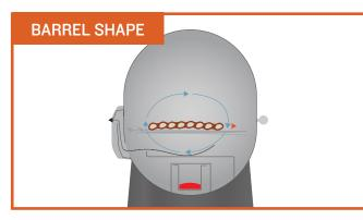
Traeger's signature barrel shape creates a vortex of convection. It circulates hot, smoky air around the cooking chamber, surrounding your food with wood-fir heat for even cooking on all sides.
