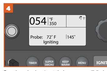
Once the probe alarm is set, the home screen will display the grill temperature, goal probe temperature, and grill status. A tone will sound when your meat reaches the set alarm temperature. If using the Traeger WiFIRE® app you will receive a push notification on your connected smart device, along with a display of your grill's status throughout the cooking process.
