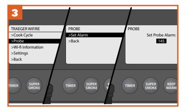
Press MENU; then scroll and select PROBE. You will be prompted to set a probe alarm for the internal goal temperature. Select SET ALARM. Then, at the probe menu, use the Selection dial to choose the temperature goal for your meat.
