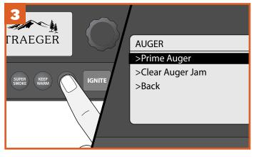
Press MENU to display the main menu. Turn the dial to select AUGER, then select Prime Auger.
