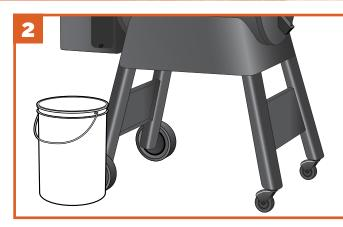
Place a container large enough to hold the discarded pellets under the pellet clean-out door.
