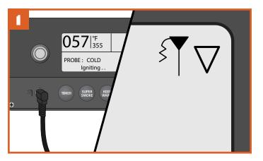
Plug the probe into the probe jack located on the WiFIRE<sup>®</sup> Controller. See "Using Your Grill" to turn on the grill. Once the grill is on, the controller will recognize the probe and the probe icon will light in the controller screen's upper-right corner.
