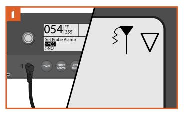
Plug the probe into the probe jack located on the WiFIRE<sup>®</sup> Controller. The controller will recognize the probe and the probe icon will light in the controller screen's upper-right corner. The display will ask if you want to set an alarm. Select YES.
