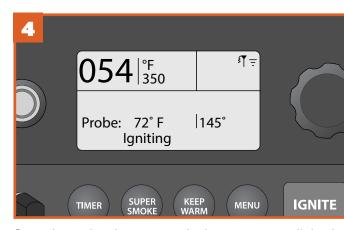
Once the probe alarm is set, the home screen will display the grill temperature, goal probe temperature, and grill status. A tone will sound when your meat reaches the set alarm temperature. If using the Traeger WiFIRE<sup>®</sup> app you will receive a push notification on your connected smart device, along with a display of your grill's status throughout the cooking process.
