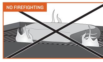
You don't have to worry about drippings flaring up and causing nasty fireballs that destroy your meal, because Traeger Wood Fired Grills cook using indirect heat. All drippings are safely channeled into an external grease bucket for easy disposal.
