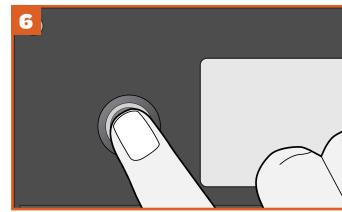
Turn off the grill by pressing and holding the Standby button for 3 seconds, initiating the shutdown cycle. Whe the full shutdown cycle finishes, seasoning of your grill i complete.
