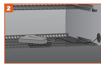
Once the grill is preheated to the desired temperature, load food into the grill. Feed the probe through the grommet on the side of the grill and insert the probe tip halfway into the thickest part of the meat—not in the fat portion or touching bone.
