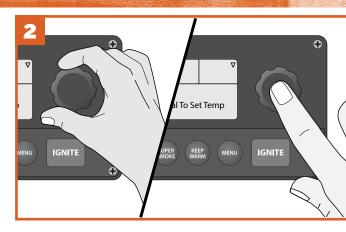
To select temperature, turn the Selection dial right or left; once the desired temperature is displayed, press the center of the dial to select.
