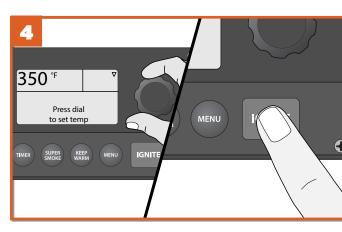
The home screen will display "Press dial to set temp." Turn the Selection dial clockwise to 350°F (177°C). Pres IGNITE, close grill door, and run grill for 20 minutes once it has reached the set temperature.
