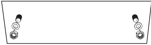
Hex Nuts/Washers attach to threaded studs Fryer Wall
