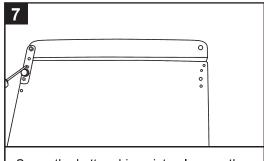
Screw the bottom hinge into place on the new side. Replace the other foot on the other side.
