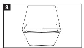
Check that the door is aligned horizontally and vertically and that the seals are closed on all sides before finally tightening the upper hinge. Re-adjust the leveling feet.
