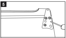
Screw the three screws to install the top bracket on top right side of appliance. Slide the appliance door back on to the top hinge. Making sure it's face up. Then replace the "plastic cover" on the top bracket by clicking back into position of door hinge.
