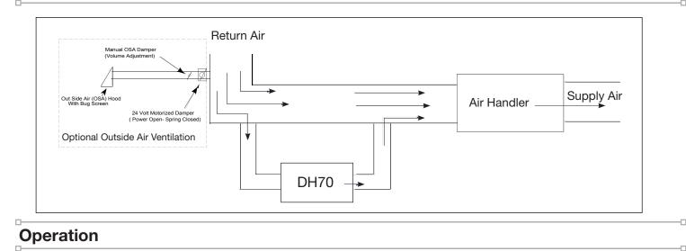
The DH70 is designed to deliver dehumidified, filtered air to the living space. It is equipped with an onboard Dehumidistat and fan control, and can be equipped with various accessories to enhance its operation (including a remote Dehumidistat).
