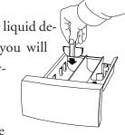
slot furthest in in the compartment as illustrated. Pour the detergent directly into the main wash compartment (2).
