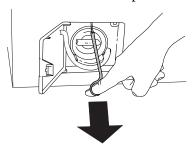
• Put the handle into its slot and screw it into place. Close the drain pump cover.
