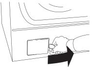
• Unscrew the screw holding the red plastic
