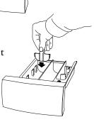
sert it in the slot furthest in in the compartment as illustrated. Pour the detergent direct into the main wash compartment (2).
