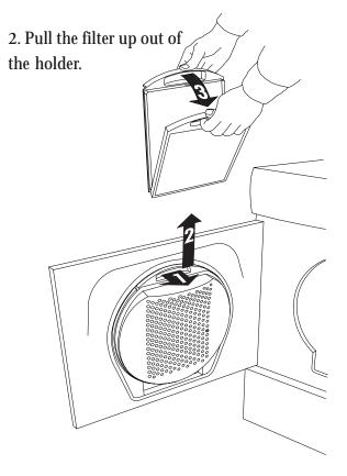
3. Open the filter and brush away the lint with your hand. Rinse the filter to remove any deposit of lime.
