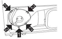
4. Unscrew the nut while holding the fan.
