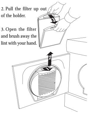
4. Fold the filter together and put it back in the filter holder.
